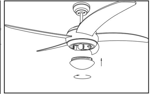
Carefully install the glass shade into the main body and turn it clockwise to lock it.
