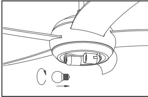
Insert-2-E27 Max.40W light bulb mounted on lamps.
