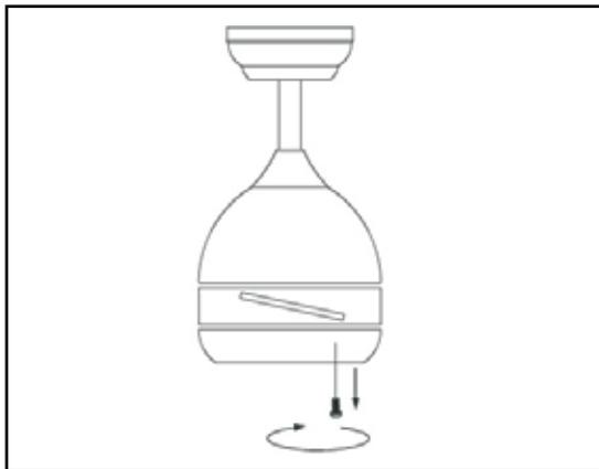
Removed the 3 screws & the lamp holder from the fixing panel.
