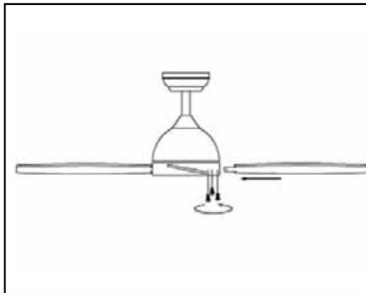
Insert the blades through the motor housing's side slots and align them with the 3 holes.
