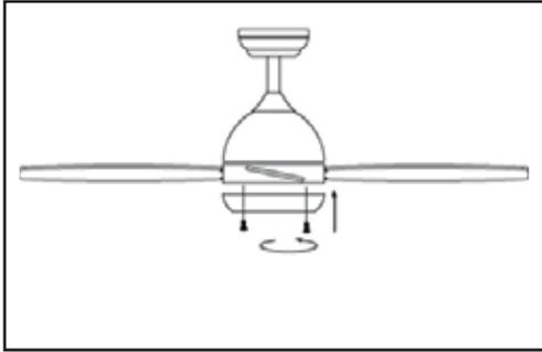
Align the lamp holder's screw holes with those on the motor and attach both parts by means of the screws provided.
